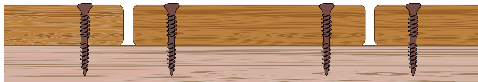
installation with visible screws
