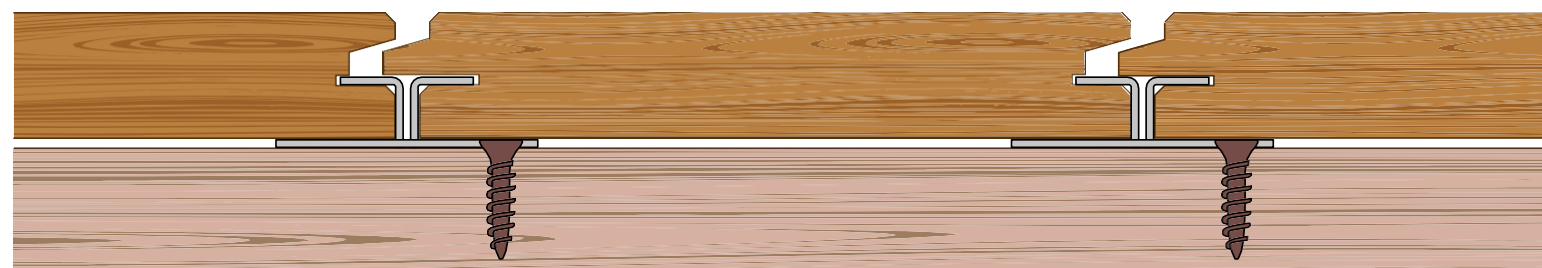
installation with concealed milling
